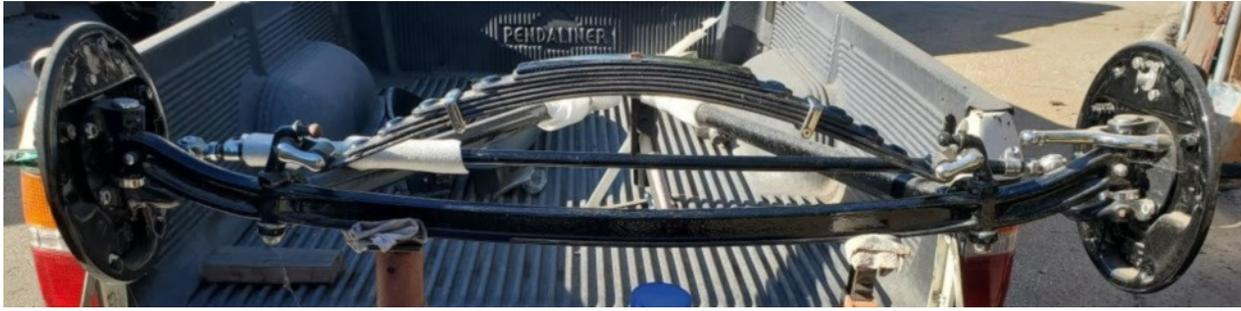
Black powder coat and Stainless Steel hardware dress it up a bit. The spring from Posey's has reversed eyes. I took the car to Bent Customs and had all new brake lines fabricated. They are a work of art.
