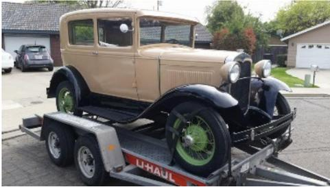
The first thing I did was to take it to Jack's and get the top installed. Then the Green wheels were replaced with a set of Tacoma Cream 1935 16" wheels. I had the rear wheels widened 1.5" so the 750x16 tires would fit better. 600x16s bring the front end closer to the ground. A "High
