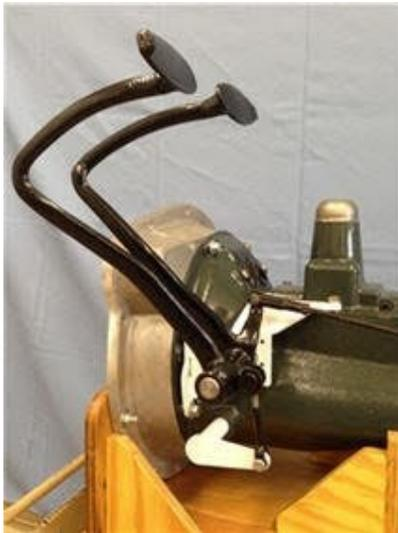
I had the Diamond block engine rebuilt at Turlock Machine. Inserted bearings, "B" Crank, Custom oil pump and full pressure oiling, topped off with one of Charlie Yapp's Riley heads. A Weber carburetor feeds the engine. Lightened flywheel with V8 clutch. Jim Birely's cam opens the valves. The re-builder estimates it will put out 85 HP.
